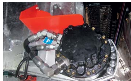
Top radial piston hydraulic motor
