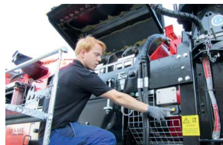
Top rotor cover – can be lifted hydraulically
