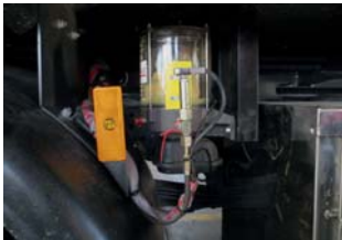
Central lubrication – fill level indicator on the process box
