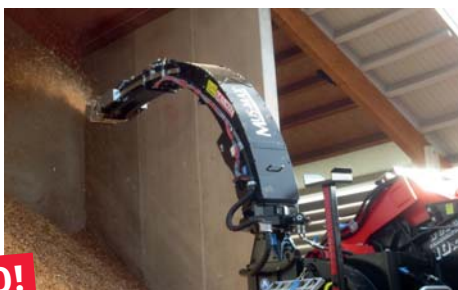
Blowing upwards with ejector is possible
