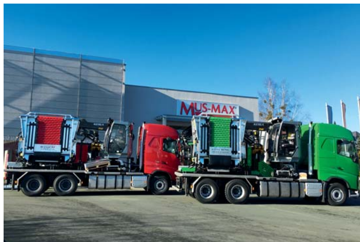
Hack Truck Volvo WT 10XL and WT 11 (up to 750 hp) with RBV intermediate gearbox
