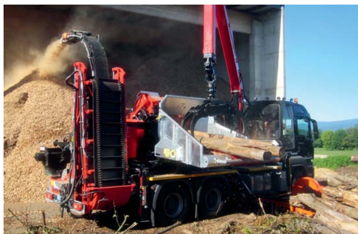
Wood chip discharge with blower
