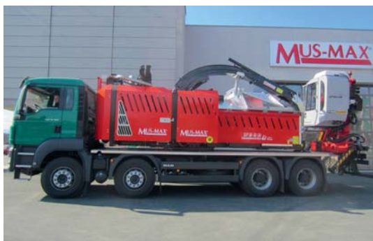
Hacker on saddle vehicle, can be swivelled left and right, with built-up wood splitter
