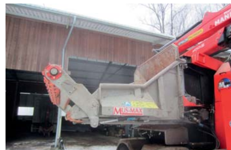
Top extension panel, hinged – feed length: 3.15 m
