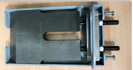
Top chopping knife setting gauge: quick blade change
