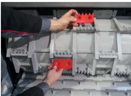
Crock System: Exchangeable knives and tines
