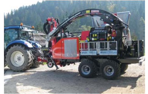
WT 9 XL DS on trailers with a 380 hp Mercedes diesel engine
