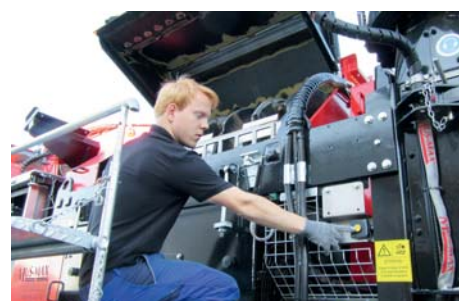
Top rotor cover – can be lifted hydraulically
