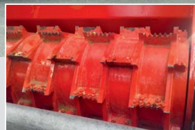
Croc system: quick exchange of knives and tines
