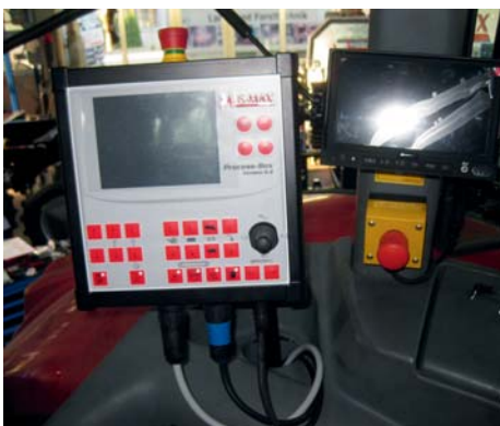
Process box and emergency stop for crane
