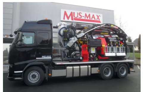
Hack truck WT 9 XL RBV with transmission from the main drive
