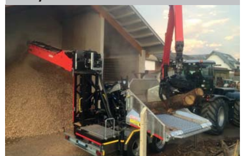
WT 11 for tractor with ascending conveyor and discharge conveyor
